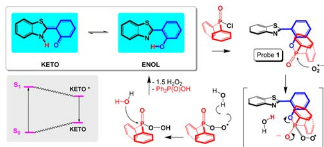
Figure 3. Synthesis of probe 1 from 2-(benzothiazol-2-yl)-phenol (HBT), its deprotonation, and a depiction of the ESIPT mechanism involving plausible ROS-based byproducts.
